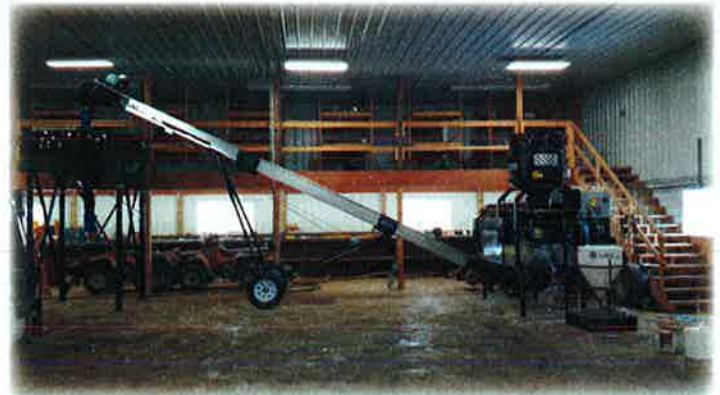
Quality Grain Services' new USC LPX 2000 seed treater, conveyor and surge hopper system.
